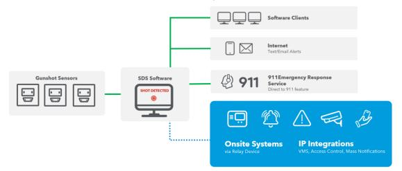
Our library of certified third-party integrations enable us to automatically trigger video, mass notification, access control, onsite alarms, emergency lighting and more in reaction to shots detected by the SDS Indoor Gunshot Detection System.
